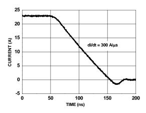
Figure 14. FDMS2510SDC SyncFET body diode reverse recovery characteristic
