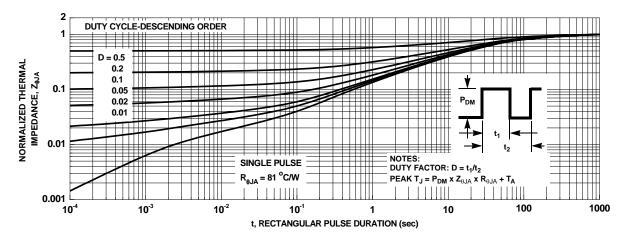
Figure 13. Junction-to-Ambient Transient Thermal Response Curve
