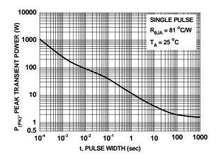
Figure 12. Single Pulse Maximum Power Dissipation
