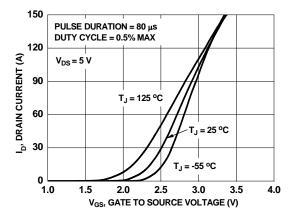
Figure 5. Transfer Characteristics
