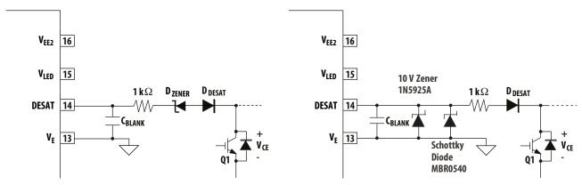
Figure 27. DESAT diode and DESAT threshold
