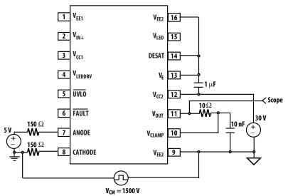
Figure 16. CMR  $V_{OUT}$  High test circuit
