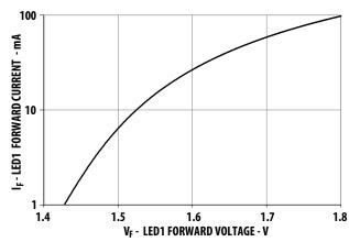
Figure 4. LED1 Input Current vs. forward voltage
