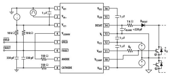
Figure 22. Typical gate drive circuits with DESAT detection
