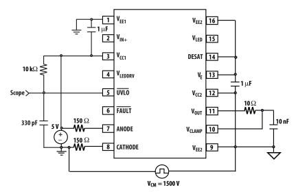
Figure 21. CMR UVLO Low test circuit
