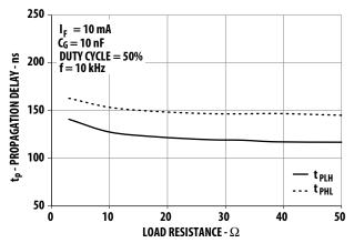
Figure 15. Propagation delay vs. load resistance
