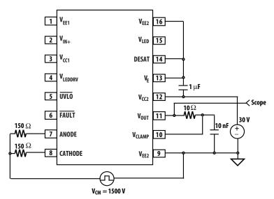
Figure 17. CMR  $V_{OUT}$  Low test circuit
