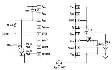
Figure 20. CMR UVLO High test circuit
