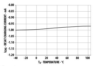
Figure 11. I<sub>CHG</sub> vs. temperature
