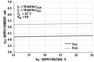
Figure 3. I<sub>CC</sub> vs.V<sub>CC</sub>
