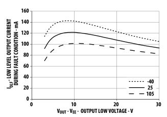
Figure 9. I<sub>OLF</sub> vs. output voltage
