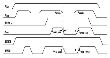
Figure 24. UVLO and feedback behaviors and timing diagram
