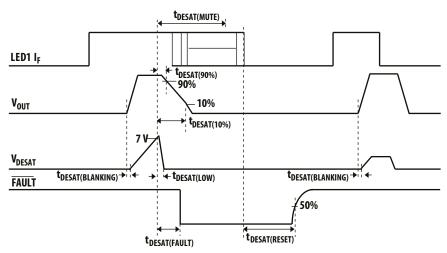
Figure 26. DESAT fault state timing diagram
