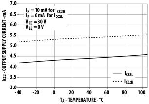
Figure 2. I<sub>CC2</sub> vs. temperature
