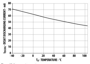
Figure 12. I<sub>DSCHG</sub> vs. temperature
