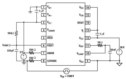
Figure 19. CMR FAULT Low test circuit
