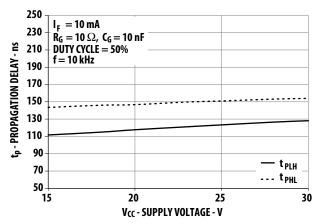
Figure 14. Propagation delay vs. supply voltage
