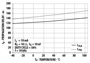
Figure 13. Propagation delay vs. temperature
