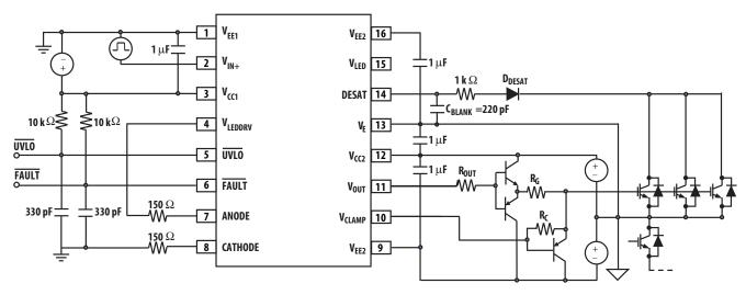
Figure 23. Typical parallel IGBT gate drive circuits with DESAT detection
