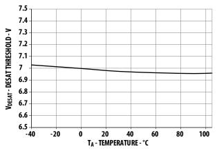
Figure 10. V<sub>DESAT</sub> vs. temperature
