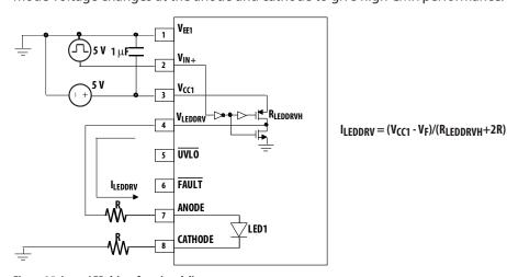
Figure 25. Input LED driver functional diagram
