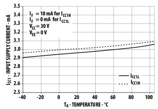
Figure 1. I<sub>CC1</sub> vs. temperature
