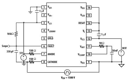
Figure 18. CMR FAULT High test circuit
