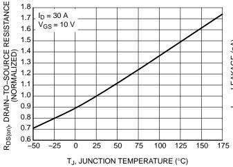
Figure 5. On–Resistance Variation with Temperature
