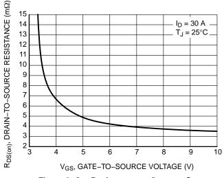
Figure 3. On-Resistance vs. Gate-to-Source Voltage
