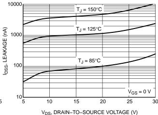
Figure 6. Drain-to-Source Leakage Current vs. Voltage
