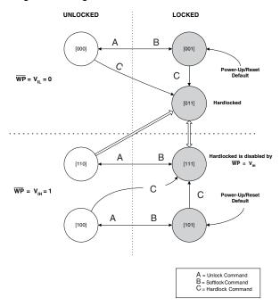
Note: 1. The notation [X, Y, Z] denotes the locking state of a sector. The current locking state of a sector is defined by the state of  $\overline{\text{WP}}$  and the two bits of the sector-lock status D[1:0].
