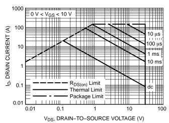
Figure 10. Maximum Rated Forward Biased Safe Operating Area
