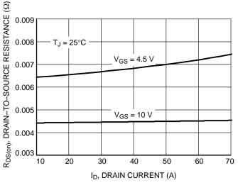
Figure 3. On-Resistance vs. Gate-to-Source Voltage
