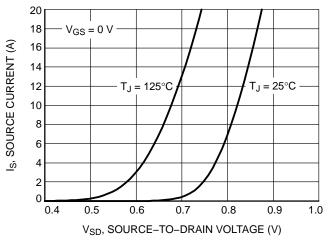
Figure 9. Diode Forward Voltage vs. Current
