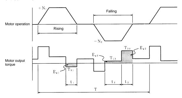
**Note** In the output torque graph, acceleration in the positive direction (rising) is shown as positive, and acceleration in the negative direction (falling) is shown as negative.
