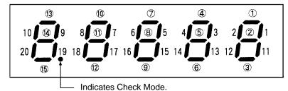
The vertical LEDs show the ON/OFF status of inputs (1 to 20) and the horizontal LEDs show the ON (lit)/OFF (not lit) status of outputs ((1) to (15)).
