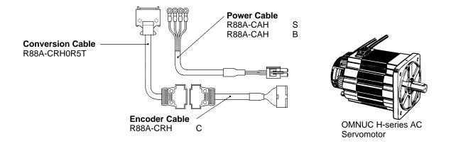
Note Refer to Chapter 5 Specifications for connector and cable specifications.
