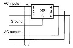
• Use twisted-pair cables for the power supply cables whenever possible, or bind the cables.
