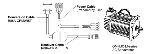
Note Refer to Chapter 5 Specifications for connector and cable specifications.
