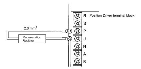
**Note** With the FND-X50H- , connect a Regeneration Resistor between P and JP1. In this case, remove the short bar between JP1 and JP2.
