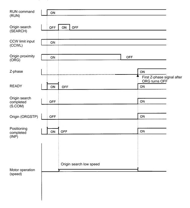
**Note** After the RUN command (RUN) signal turns ON, there will be an interval of 110 ms max. before the READY signal and the positioning completed (INP) signal turn ON.
