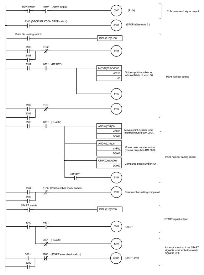
**Note** 1. The point number setting switch is a contact for taking the point number (DM 00) into the Position Driver.
