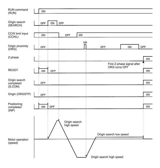
**Note** After the RUN command (RUN) signal turns ON, there will be an interval of 110 ms max. before the READY signal and the positioning completed (INP) signal turn ON.
