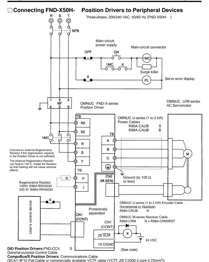
Note When using the CompoBus/S Position Drivers, create the same sequence using the ALM bit.
