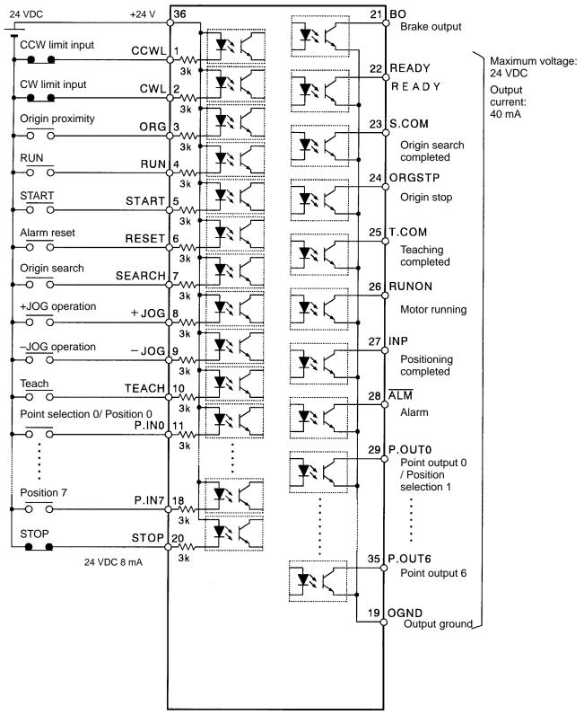
**Note** 1. The wiring for control inputs P.IN 1 to 6 is omitted. The input circuitry is the same as for P.IN0.
