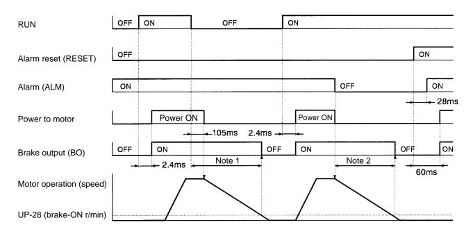
**Note** 1. When the motor is stopped, the brake output turns OFF in approximately 2.4 ms.
