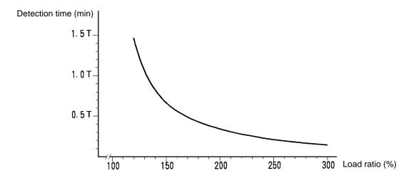
**Note** 1. The load ratio is calculated in relation to the motor's rated current.
