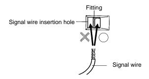
3. Tighten the cable terminal block screws to the proper torque of 0.5 N m for each signal wire. Use a small flat-head screwdriver with of uniform thickness. A normal screwdriver which is thin only at the end will not fit all the way in.
