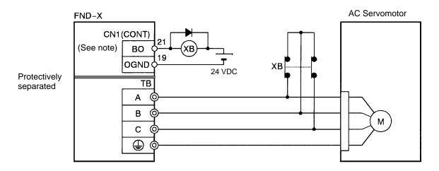
**Note** With the CompoBus/S Position Drivers, outputs are made to CN4 (LIMIT). BO (CN4 to 8) and OGND (CN4 to 14) are provided. For controlling dynamic brake drive bits, use the CN4 to CN8 pin outputs.
