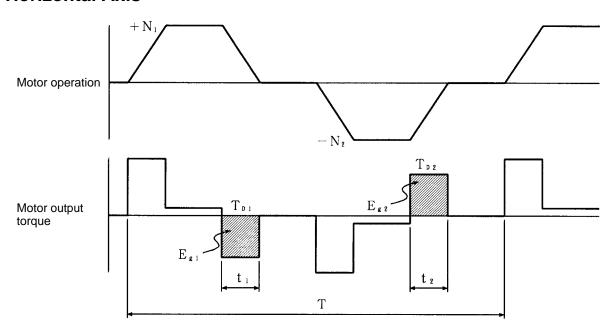
**Note** In the output torque graph, acceleration in the positive direction is shown as positive, and acceleration in the negative direction is shown as negative.
