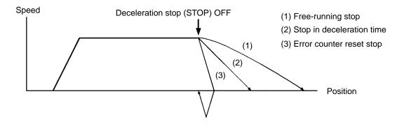
**Note** After the deceleration stop (STOP) signal turns OFF, there is a maximum delay of 1.6 ms before the stop processing begins.
