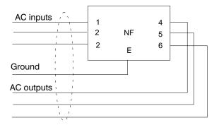
• Use twisted-pair cables for the power supply cables whenever possible, or bind the cables.
