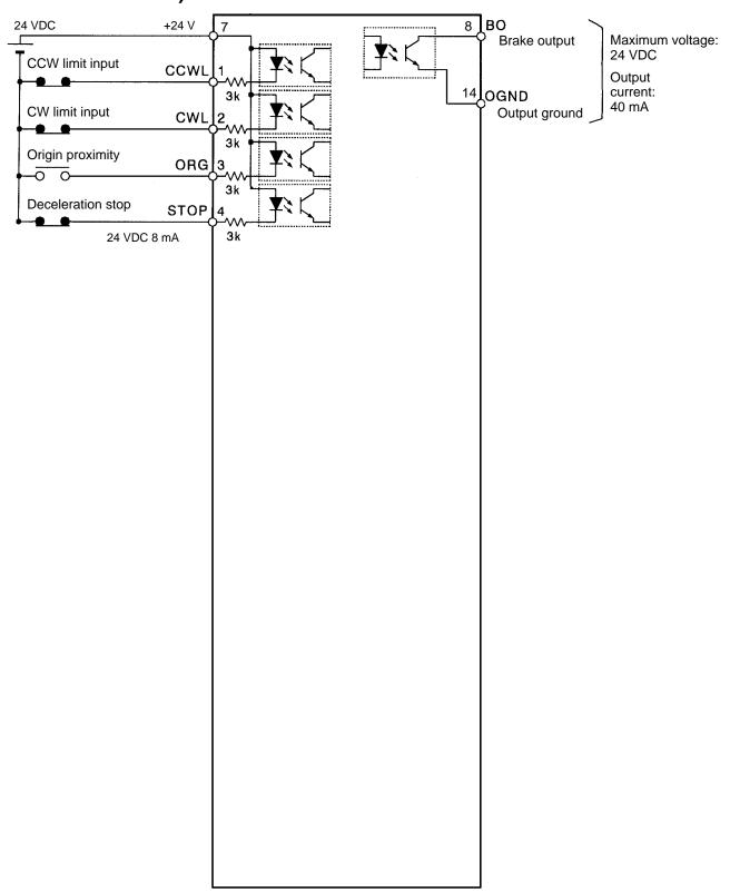
**Note** The Servomotor cannot be driven if the deceleration stop signal if OFF for the external control input (CN4-4) or the CompoBus/S input (OUT7).
