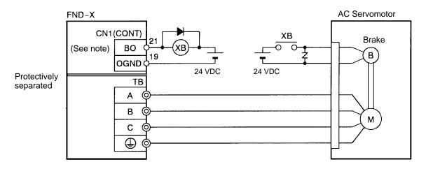
**Note** With the CompoBus/S Position Drivers, outputs are made to CN4 (LIMIT). BO (CN4 to 8) and OGND (CN4 to 14) are provided. For controlling brake drive bits, use the CN4 to CN8 pin outputs.
