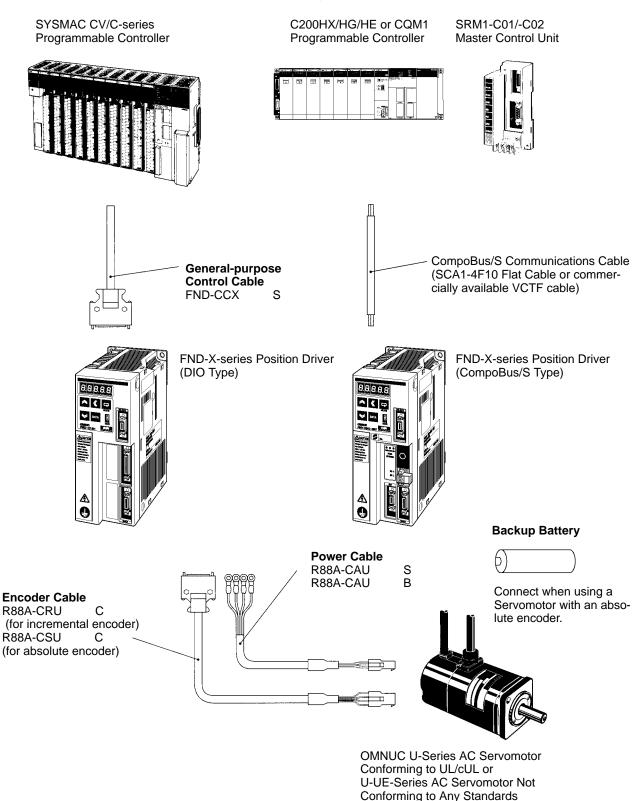
**Note** Refer to *Chapter 5 Specifications* for connector and cable specifications.
