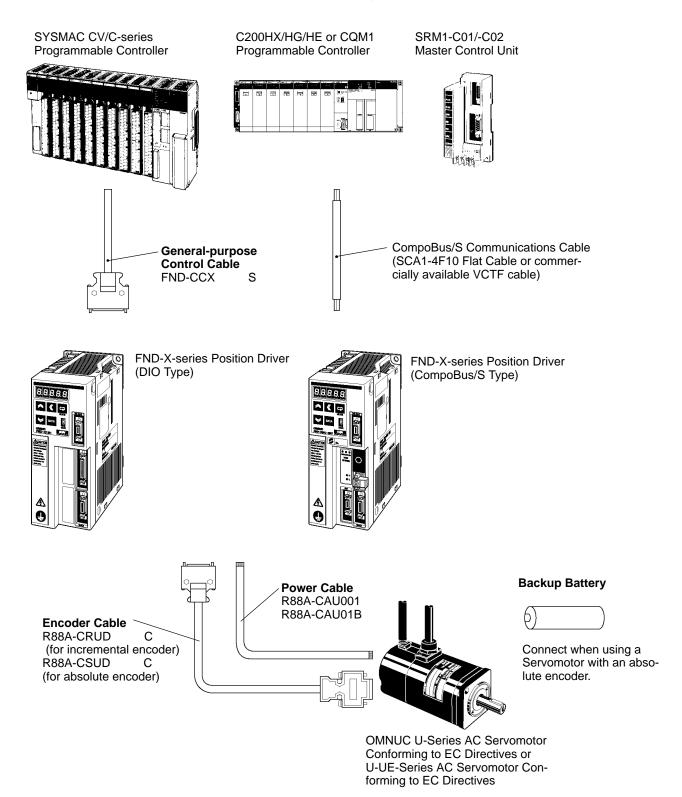
**Note** Refer to *Chapter 5 Specifications* for connector and cable specifications.
