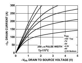
Figure 10. Saturation Characteristics
