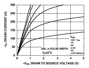
Figure 9. Saturation Characteristics
