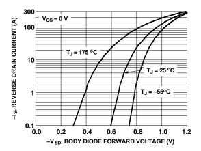
**Figure 8. Forward Diode Characteristics**
