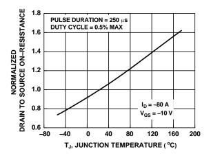
Figure 12. Normalized R<sub>DS(on)</sub> vs. Junction Temperature
