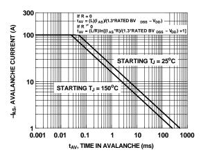
Figure 6. Unclamped Inductive Switching Capability
