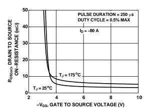
Figure 11. R<sub>DS(on)</sub> vs. Gate Voltage
