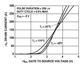
**Figure 7. Transfer Characteristics**
