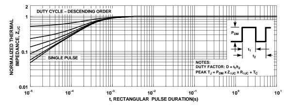
Figure 3. Normalized Maximum Transient Thermal Impedance
