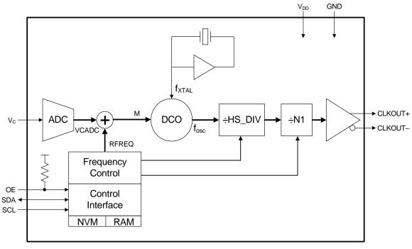
Figure 2. Si571 Detailed Block Diagram
