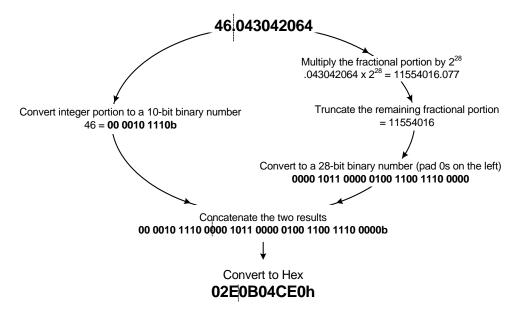
Figure 4. Example of RFREQ Decimal to Hexadecimal Conversion
