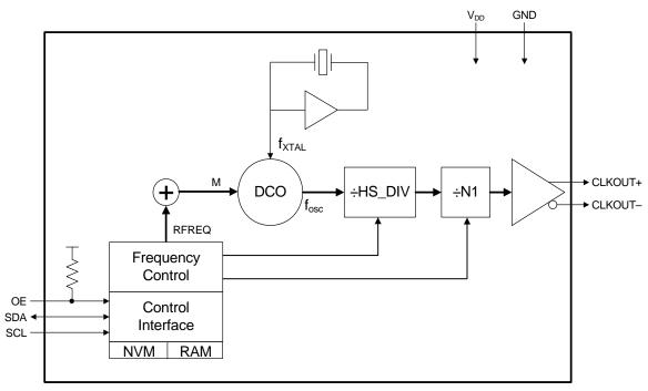
Figure 1. Si570 Detailed Block Diagram
