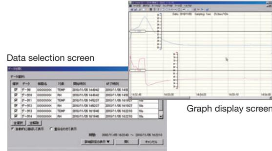
Insert the SD card containing collected data into a PC, and simply designate the drive in order to manage and graph the recorded data. Measurement data is stored in CSV format, allowing for easy temperature and humidity data management.
