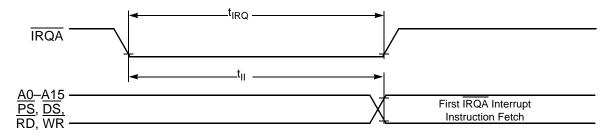
Figure 3-18 Recovery from Stop State Using IRQA Interrupt Service
