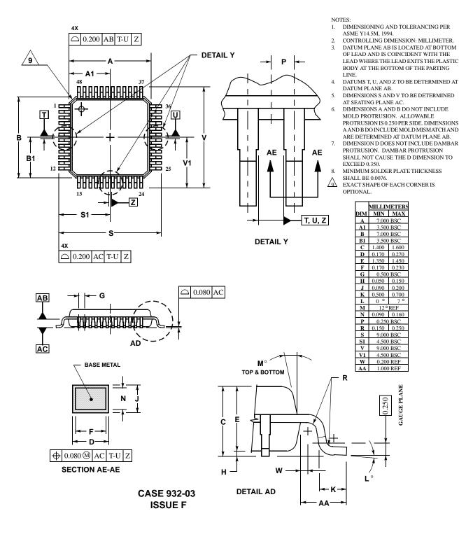
Figure 4-2 48-pin LQFP Mechanical Information
