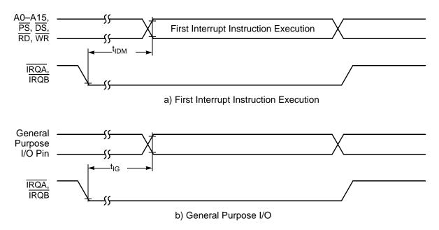
Figure 3-15 External Level-Sensitive Interrupt Timing
