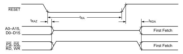
Figure 3-13 Asynchronous Reset Timing
